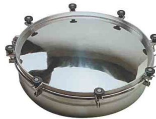
D14 Outward opening with internal Ø700/800/1000/1200/1400mm, removable sanitary double lip seal, frame size 100 x 3mm (max. pressure 0.3 bar)
