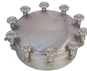
D13 Outward opening TUV certified, internal Ø300/400/450/500/600mm (max. pressure 1.5-10 bar dependant upon diameter and number of swing bolts. Also suitable for vacuum)
