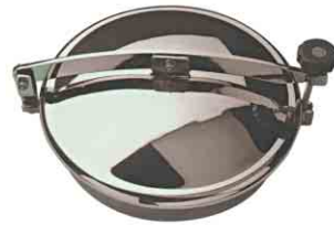
D8 Outward opening with retention free cover design and removable sanitary double lip seal, frame size 100 x 2.5mm, internal Ø200/300/420/460/500/600mm (max pressure 0.2 bar)
