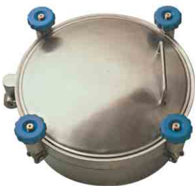
D3 Outward opening with 150 x 4mm frame, internal Ø300/400/450/500/600mm (max pressure 2-6 bar dependant upon diameter and number of swing bolts. Also suitable for vacuum)
