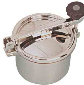
D10 Outward opening with internal Ø200mm, frame size 50 x 2.5mm, increased frame height on request (max. pressure 0.2 bar)
