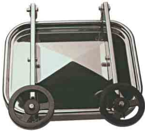
B2 Outward opening with 60 x 8mm frame, internal dimensions 530 x 410mm (max. pressure 1.2 bar)
