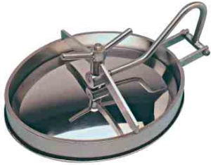
A16 Inward opening with swivel joint and 100 x 12mm frame, internal dimensions 520 x 420mm (max. pressure 6 bar). Dimensions 495 x 395mm (max. pressure 3 bar) also available
